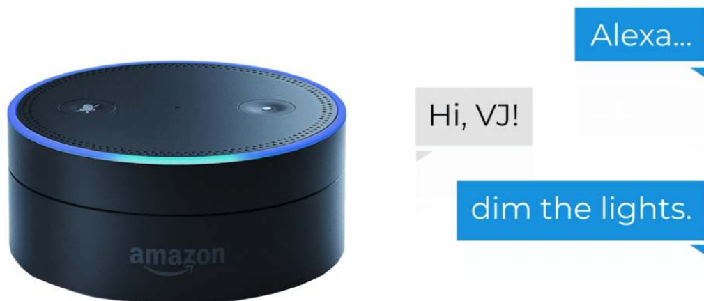
Figure 4.3: Keyword Spotting in Action: An Amazon Echo Dot responds to the wake word and follows the user’s command. Voice-activated devices use a lightweight, always-on wake-word detector that listens continuously and triggers the main voice assistant only after the keyword is spoken.
